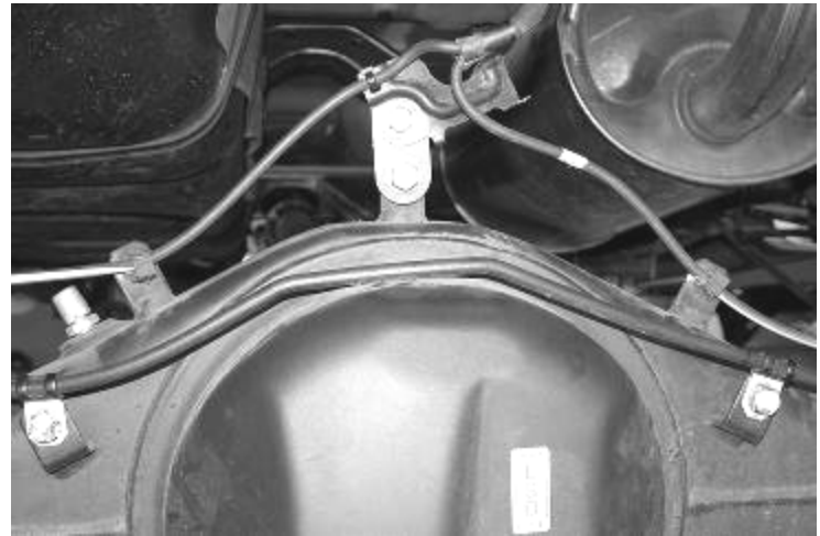
re-install A.B.S. line back into plastic clips
