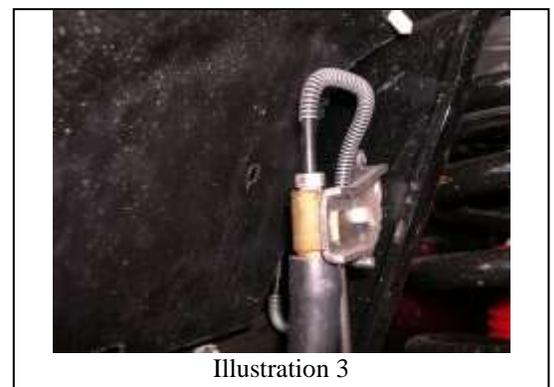
**TECH TIP:** Having someone turn the steering wheel slightly will help align track bar bolt.
