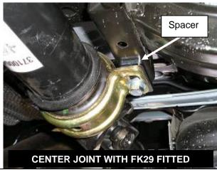
Tighten both bolts firmly.
