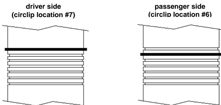
On **4x2** models, it is recommended that the **driver side circlip is installed two positions higher than the passenger side circlip**. For example, to achieve the only offered lift setting of 2.55", the circlips should be installed as follows (**Note: Do not use circlip locations #4, #5, #6, or #7 on 4x2 models**):
